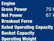
Perkins 854F-E34TAN 70 kW (94 hp / 95 ps) @ 2,200 rpm 67 kW (90 hp / 91 ps) @ 2,200 rpm 30 kN city 1,496 kg (3,300 lb) 0.55 m<sup>3</sup> 5,190 kg
